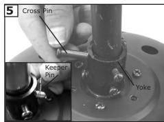
Insert downrod into yoke on top of the Fan Body. Align the hole in the Downrod with the hole in the Yoke. Insert the Pin through the Yoke and Downrod until the point appears on the other side. Install the Keeper Pin
